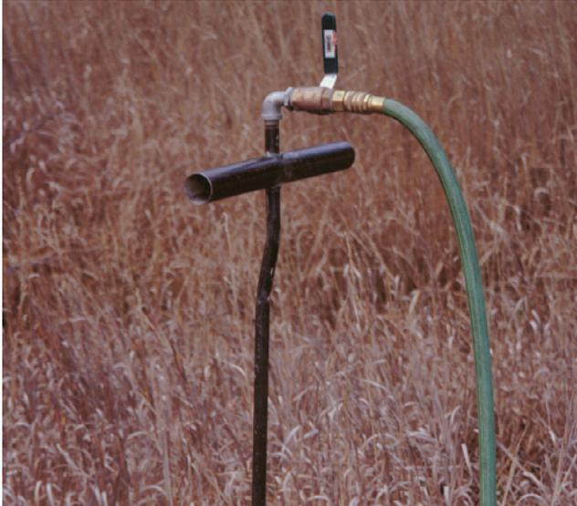
Figure C4—Handle with ball valve.
