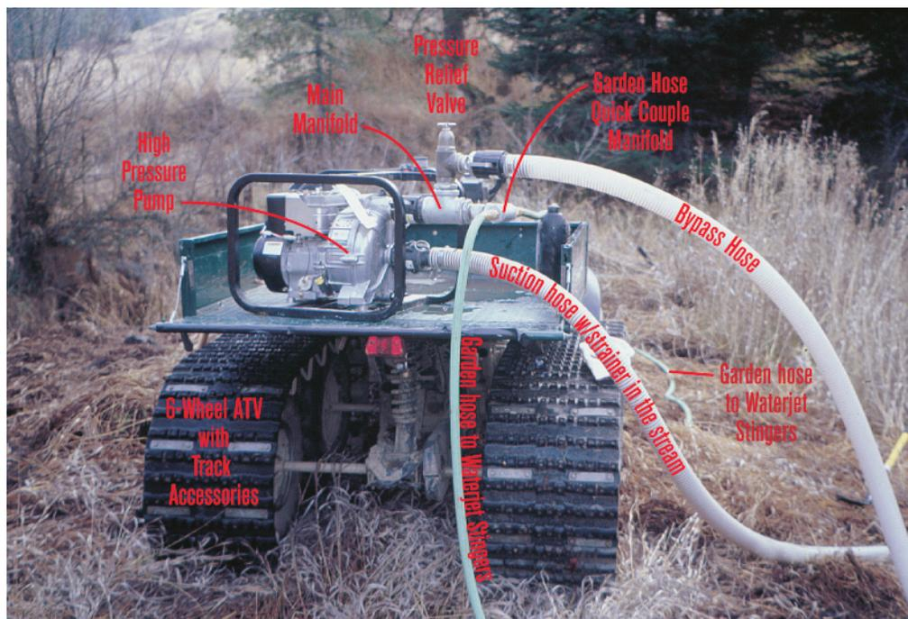
Figure C17-6-wheel ATV with track accessory
