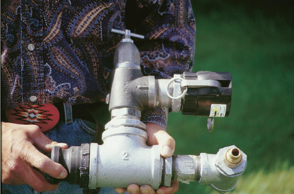
Figure C13—Waterjet Stinger manifold.
