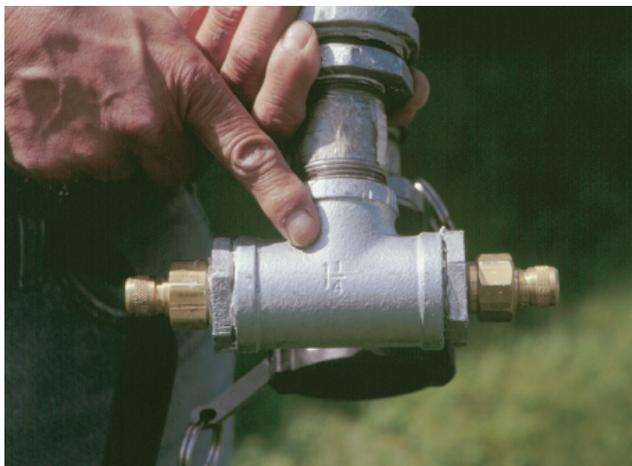
Figure C5— Garden hose quick coupler manifold.
