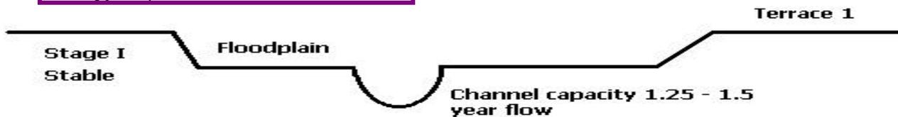
**A** Stage I channel is a stable, relatively small channel that carries water and sediment in a manner such that the stream is neither aggrading or degrading. This does not mean that Stage I streams do not change positions in the landscape. Even though a stream is considered stable, it still has the ability to adjust, and is considered to be in a state of **DYNAMIC EQUILIBRIUM**.
